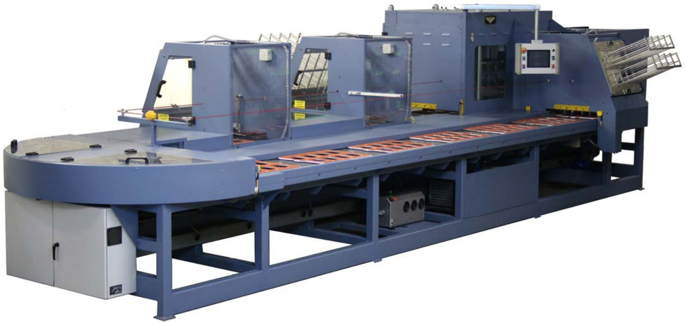
Typical BSC II Series Carousel Machine shown with three feeders and finished package unloader
