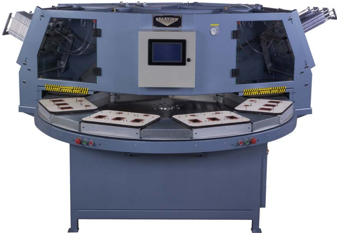
FAB Series Automatic Rotary Blister Sealing Machines Eight-station machine shown
